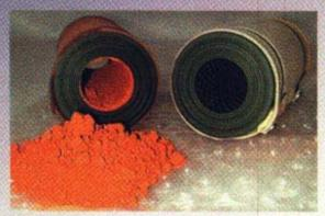
Before and after, shows one of our coalescing elements and the pipe scale and dirt it filtered out of an air line. (Coalescing flow is inside to outside) At right is a new element ready to go into service
