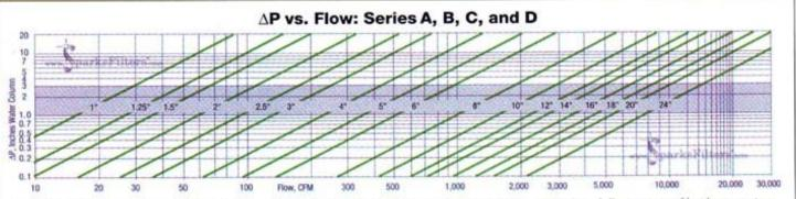
Use the chart above to access the init. AP vs. flow for series A. B. C. & D air intakes. Be aware that the maximum practical flow through a filter housing, like other piping, is limited primarily by the cross sectional area of the connection. Compare the connection size shown
